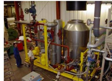
To cover with the extreme temperatures and storms (maximum wave height 12,1 meter) a stainless steel outer shell was applied for the boiler in combination with a weather resistant paint system. The skid mounted unit complies with the offshore requirements as listed by the American Bureau of Shipping (ABS). In addition electric motors and instruments have been selected in Exd and the control panel in Exp execution. With an additional human man interface (HMI) to control the unit from inside.
