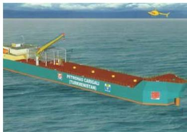
Steam is used for keeping the crude oil in the FSO’s six storage tanks above 38 °C. Important since below that temperature wax is formed. Other steam demand comes from the fresh water makers, air (duct) heaters for accommodation and machinery spaces.
