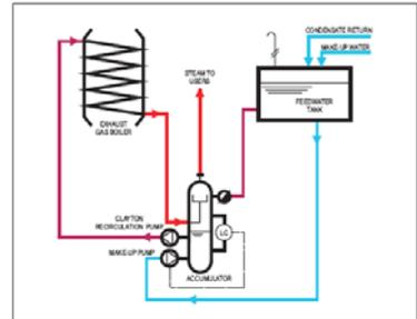
The Clayton design facilitates in drying the steam into a top quality of 99,5 % saturated steam.
