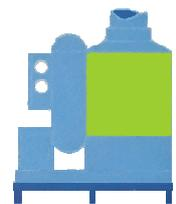
The Clayton Steam Generator can start and stop on demand and steam is produced under controlled conditions. The design used three main components which are the specially designed positive displacement pump, the heated coil and an extremely high efficiency steam separator.
